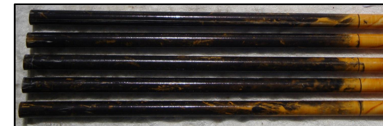
Above. Red IRIS (indicator or reduction in soils) tubes (white PVC pipes painted with iron oxide paint) become blackened after being inserted into tidal marsh soil for only a few minutes. Black areas are iron sulfide that forms rapidly by chemical reaction of dissolved H 2 S and/or HS - with the iron oxides. Such observations have led to a new model for how sulfidization takes place (paper presented at 7 th conference).
