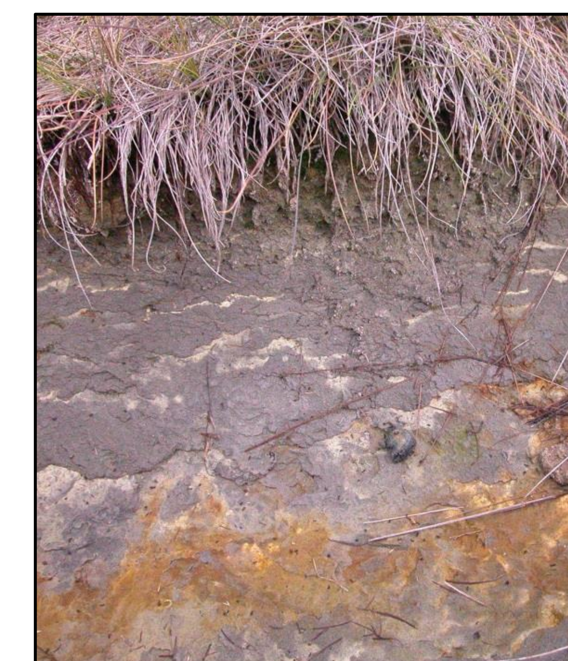
An active acid sulfate soil on a scalped land surface at Stafford Co., VA regional airport. Yellow jarosite in sulfuric horizon . Vegetation possible because of application of lime-stabilized biosolids as reclamation strategy. Web soil survey at this and other disturbed land sites often needs update as it commonly shows pre-disturbance soils not existing active acid sulfate soils, see section left corner below.
